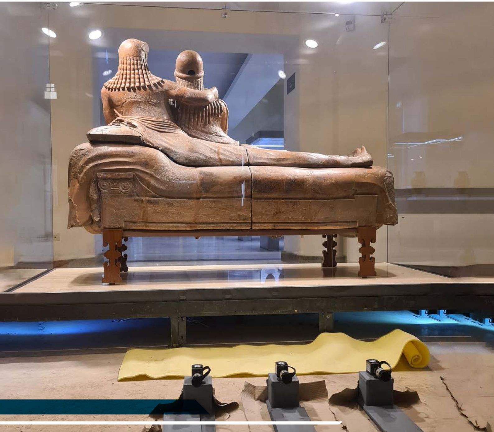
Weighing operation to verify and confirm the mass of the theca and the Sarcophagus.
