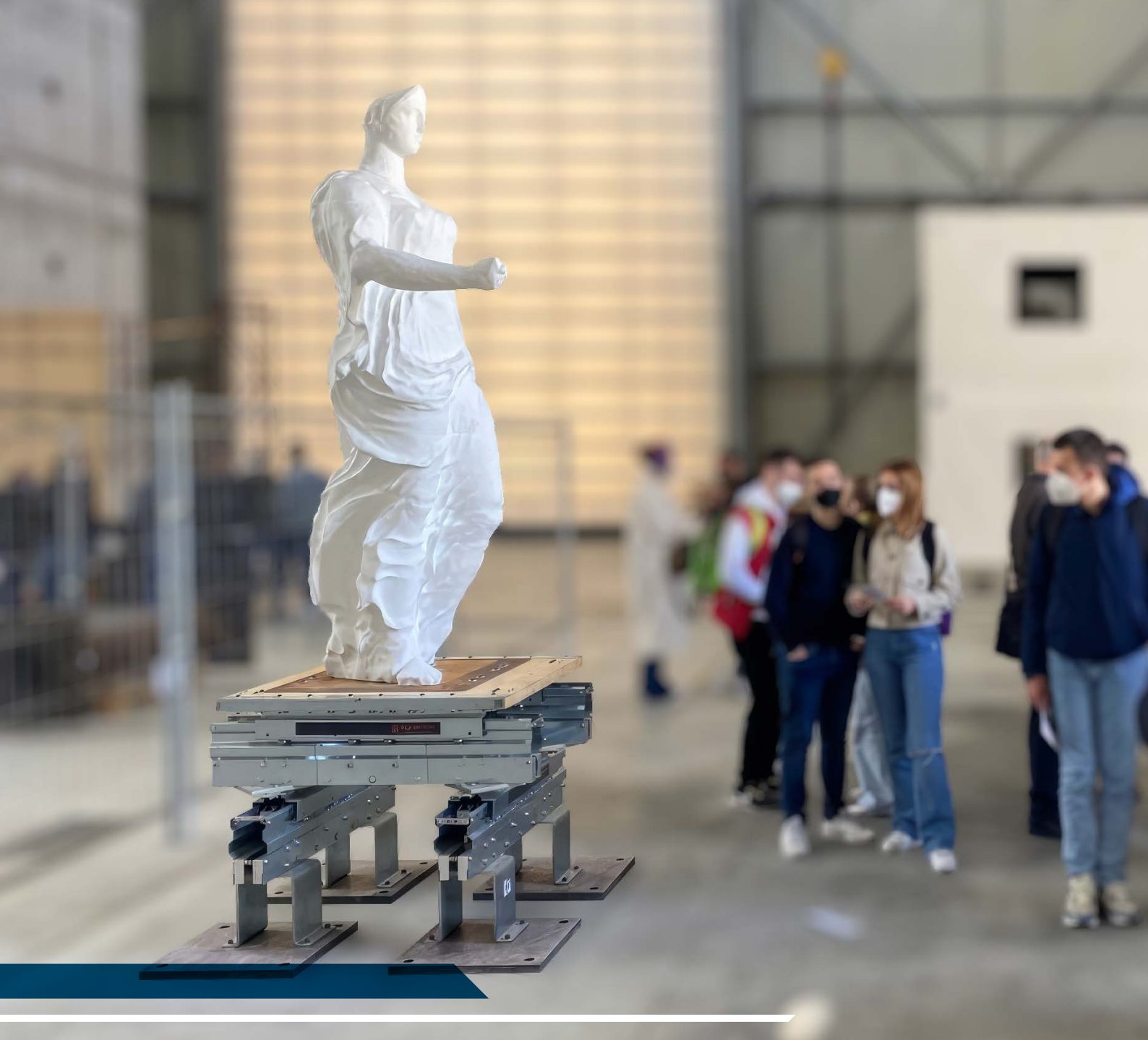
Isolation simulacrum Goddess of Morgantina. Tests carried out on the shaking table at L.E.D.A. (Laboratory of Earthquake Engineering and Dynamic Analysis – University of Enna Kore) .
